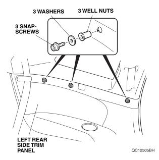
8. Place a washer onto the snap-screw and install three snap-screws into each well nut. Securely tighten the snap-screws.
