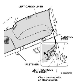
17. Attach the fastener pad to the left cargo liner as shown.
