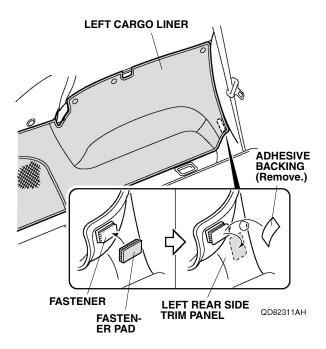
18. Remove the adhesive backing from the fastener pad, and attach the fastener pad to the left rear side trim panel.
